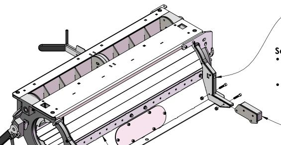
The valve bolts directly to the Romafa meter housing with M10 x 120 bolts.
